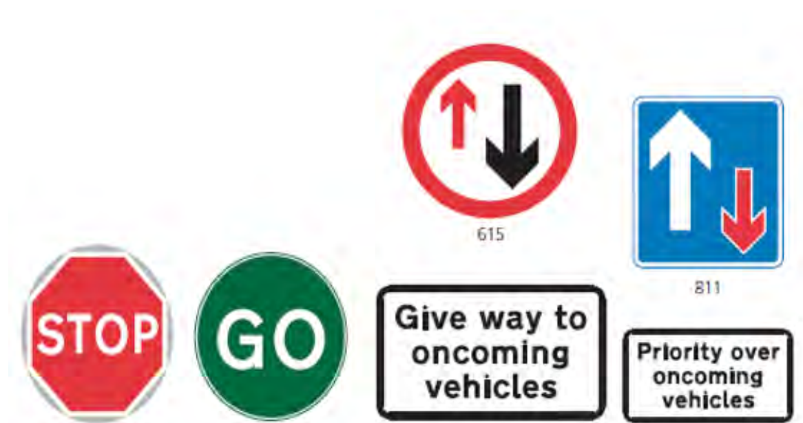
Figure 1.5: Manually operated stop/go signs and priority signs
